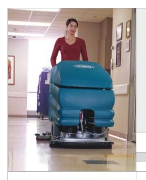
**High productivity with gel batteries.** Achieve up to 6 hours of run-time with environmentally-preferable sealed batteries.
